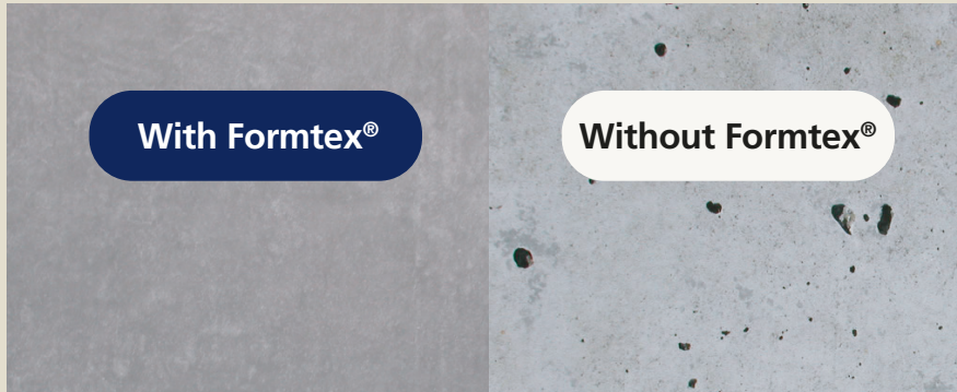
Formtex® drains surplus water and air, providing for a denser concrete cover layer without blowholes. The result is increased resistance to degradation from penetration of chloride, water, carbon dioxide and frost/thaw.
