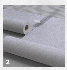
The rolls must be laid with tight joints and the joints sealed with 5 cm wide tape to prevent intervening of concrete. A thin layer of plastic foil is placed on top of the fabric, before concrete is poured.
