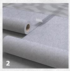
The rolls must be laid with tight joints and the joints sealed with 5 cm wide tape to prevent intervening of concrete. A thin layer of plastic foil is placed on top of the fabric, before concrete is poured.
