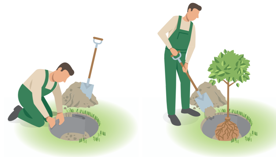
Fibertex RootSeal Premium is easily installed vertically along the edge of the hole.
