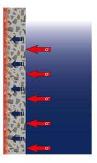
As in other porous materials capillary rise is also a transport mechanism. This is best understood by thinking of what happens when a sugar lump is held only with its lower part in a fluid. The fluid will rise through pores of the sugar lump until it is saturated. The speed of permeation and capillary rise is dependent on the denseness of the concrete.
