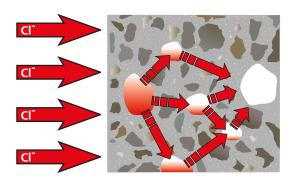
The rate of ingress will depend on the chloride concentration at the surface, and the diffusion coefficient of the concrete. The diffusion coefficient is a material property describing the speed of diffusion through the concrete. The size of the diffusion coefficient is highly dependent on the pore-structure and the denseness of the concrete and therefore mainly varies with the w/c-ratio, cement content, pozzolan content, presence of micro-cracks and curing conditions.
