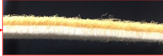
FIGURE 3 – EXAMPLE OF GSC NATURAL MARINE VEGETATION AND CROSS-SECTION PHOTOGRAPH OF THE COMPOSITE GEOTEXTILE MATERIAL (V INDEX)
