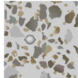
2. Corrosion of the re-bar causes expansion, and the concrete starts to crack internally.
