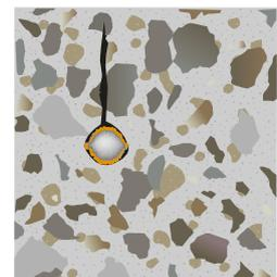
3. Corrosion continues and the cover spalls off as a result of the volume increase.
