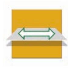
Required length of the reinforcement after failure plane for resisting direct sliding over reinforcement
