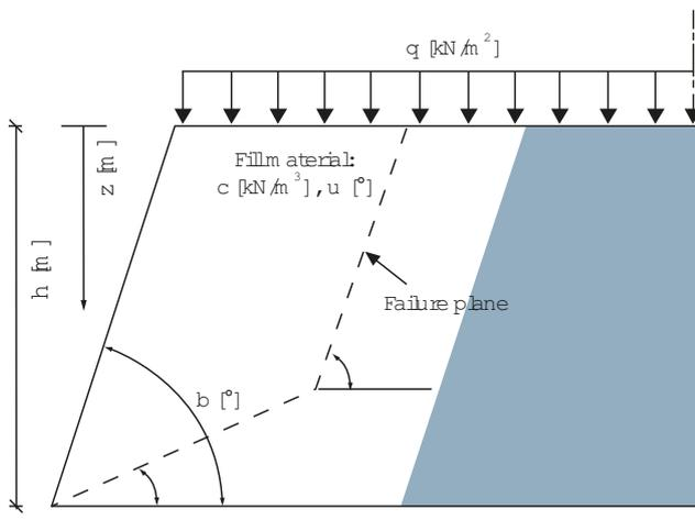
Fig 15. Reinforced slope
