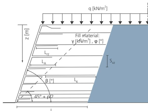
Figure: 6 Reinforcement spacing and length
