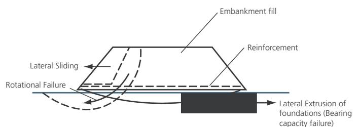
Figure: 1 Typical Failure mode for an embankment
