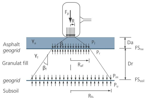
Figure: 2 Forces on the pavement
