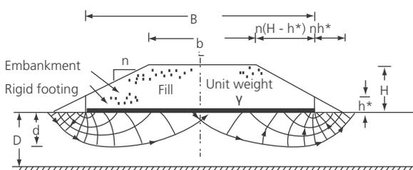
Figure: 2 Embankment on soft soil
