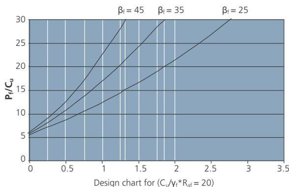
Figure: 3 Chart for designing the depth of the fill layer
