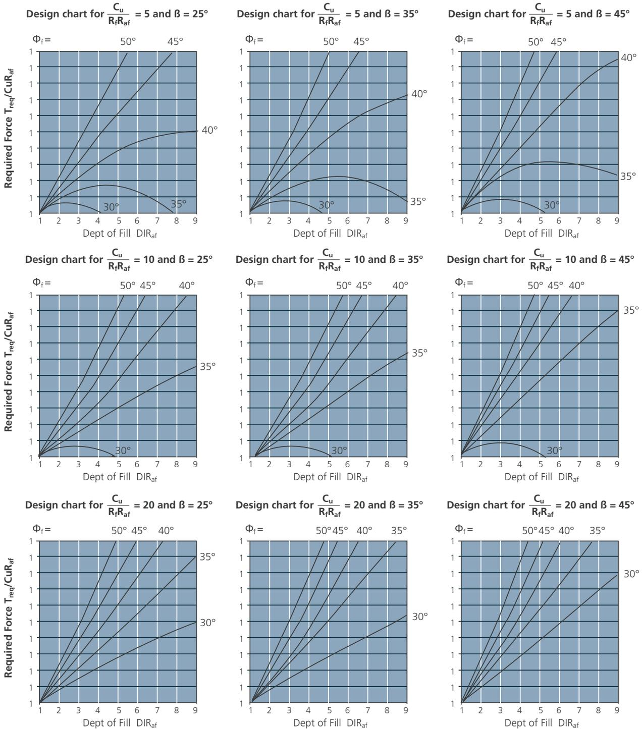
Figure: 4 Charts for tensile force in reinforcement
