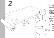
Unroll Formtex® onto the formwork.
