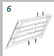
Tension tightly across the formwork using rubber hooks.
