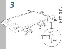
Staple the Formtex® along the bottom of the formwork while pulling it towards the sides.
