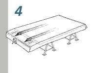
Manually tighten the liner while stapling it to the span beam.
