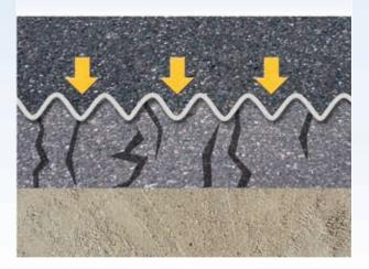
The top layer of the existing surface was milled off to create the optimal basis for the new asphalt wearing course. Fibertex AM-2 was placed on top of the deep milling cuts.
