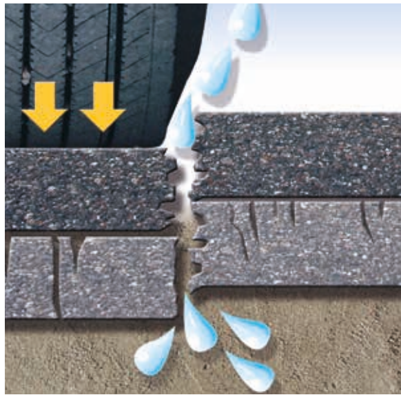
Fig. 2. Without paving fabric, reflective cracking of the new asphalt overlay will occur and surface water will enter the old asphalt layer. This will accelerate deterioration of the entire road construction.
