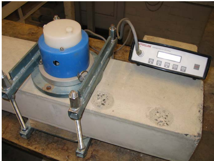
Fig. 7 The Autoclam Permeability System attached to the test block
