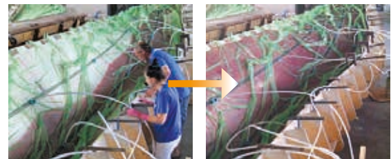
Infusion of hull using Compoflex® SB RF
