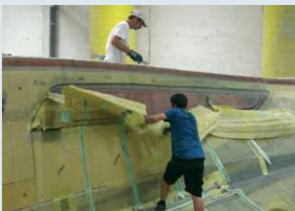
11. Minimum resin dust when removing Compoflex® RF 3.
