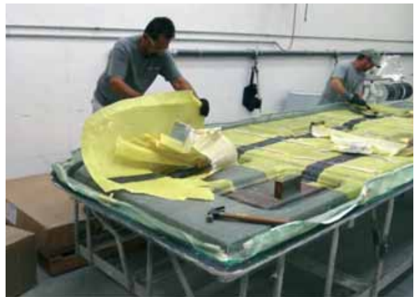
8. Easy removal of Compoflex® RF 3.
