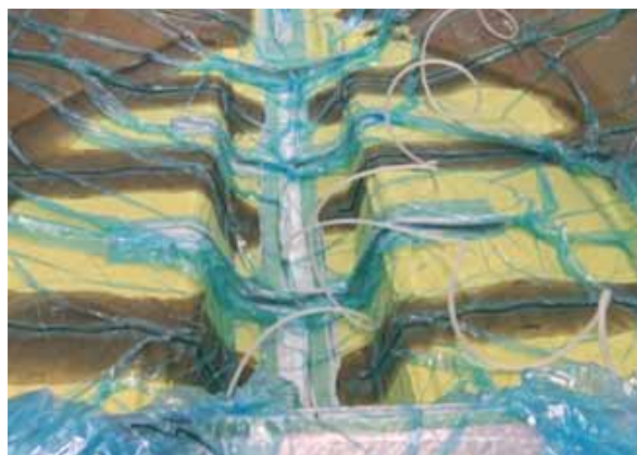
8. Even Flow with Compoflex® RF 3 helps avoid dry spots.
