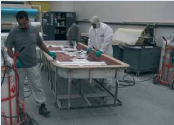
1. Lay-up of the swim platform.
