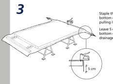
Staple the Formtex® along the bottom of the formwork while pulling it towards the sides.
