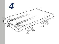
Manually tighten the liner while stapling it to the span beam.
