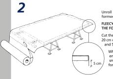
Unroll Formtex® onto the formwork.
