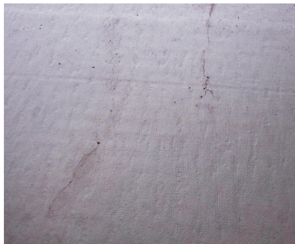
Figure 7. Several cracks in the surface of the test of the competing product.
