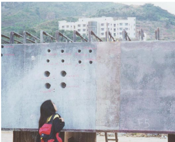
Figure 2. The trial beam, with the competing product (left), without formliner (middle) and Formtex ® (right).
