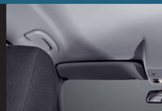
Headliners - Mouldable nonwovens offer a soft facing, acoustic control, reduced weight and a strong backing.
