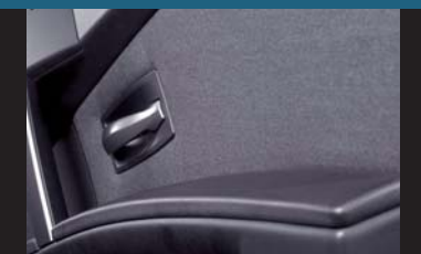
Door trim panels - Unique insulation material protects face fabric during back-injection moulding.
