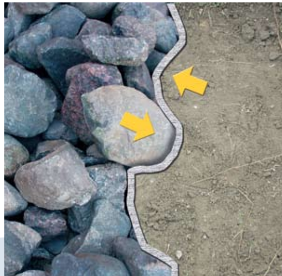
Fig. 8. High elongation allows the geotextile to follow the contours of the irregular construction surface.
