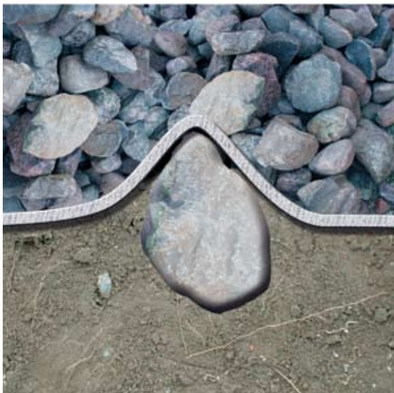
Fig. 5. High elongation and static puncture resistance allow the geotextile to stretch around the irregular construction surface.
