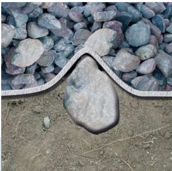
Fig. 3. High elongation and static puncture resistance allow the geotextile to stretch around the irregular construction surface.
