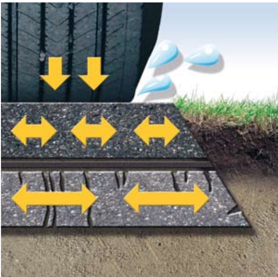
Fig. 1. The paving fabric absorbs differential movements in the asphalt layers preventing reflective cracking. Additionally it forms a waterproof interlayer preventing surface water from entering the old asphalt layer.
