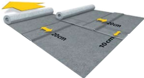
Fig. 7. A sufficient overlap in both longitudinal and transverse direction is recommended.
