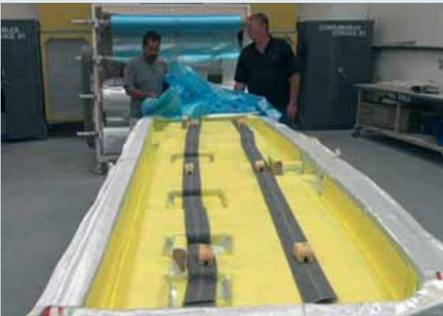
3. 510 Fly swim platform ready for bagging after Compoflex® RF 3 has been installed.
