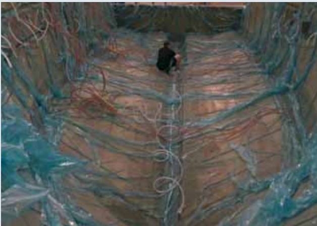
9. Infusion of the Sea Ray 510 Fly takes less than 45 minutes with the use of Compoflex® RF 3.
