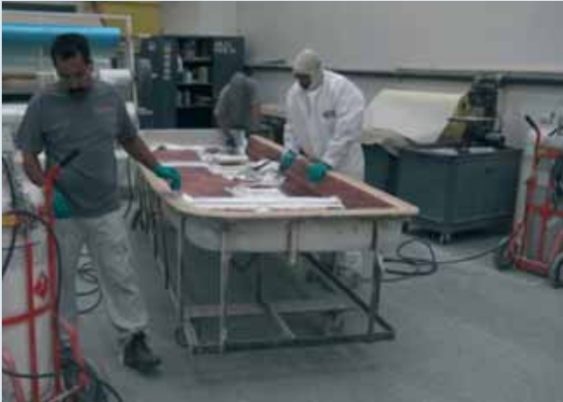
1. Lay-up of the swim platform.
