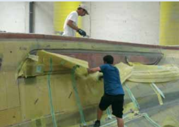
11. Minimum resin dust when removing Compoflex® RF 3.
