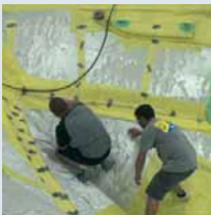
5. Compoflex® RF 3 is a genuine three-in-one product, and it is very durable when you need to climb on it during installation of flow channels and vacuum lines.
