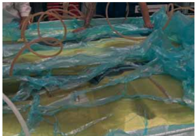
6. Infusing the whole 510 Fly swim platform takes only a few minutes.
