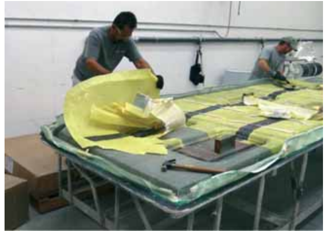
8. Easy removal of Compoflex® RF 3.
